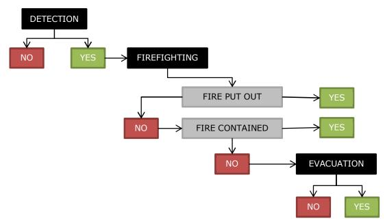
Fig.1 – Functional relationship among the 3 sub-systems within the "fire safety" system
